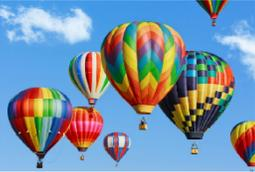
A hot air balloon has three parts: the envelope, the basket, and the burner. The burner heats the air that fills the balloon. Since hot air is lighter than cool air, the balloon floats up. The envelope is made of nylon. It can have many patterns on it. People ride in the basket below the balloon.
